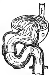
Fig. 192. Buckland & Rees's Hopper-Closet. a, Bowl. b, Trap. c, Fan. f, Supply.
